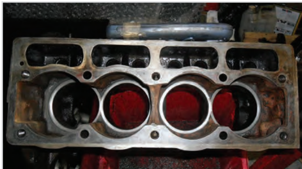
Wet Liners removed & Fig of 8 seats cleaned
